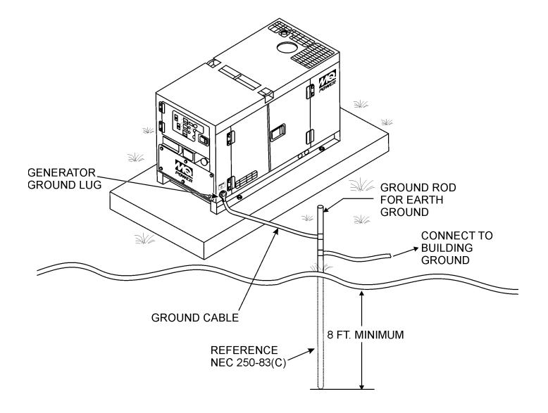
Figure 4. Typical Generator Grounding Application
